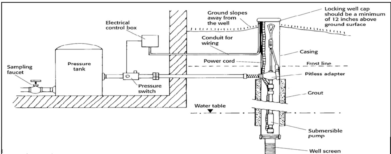
**Figure 3-2.** A properly constructed well.
