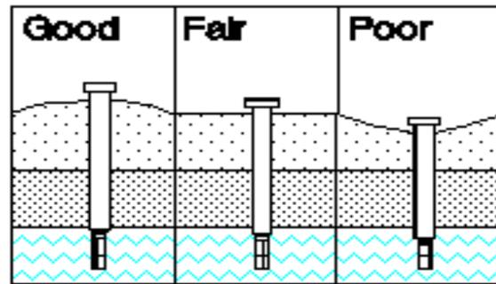
**Figure 3-3.** Comparison of well placements at ground surface. With proper placement, ground surface will slope away from well.
