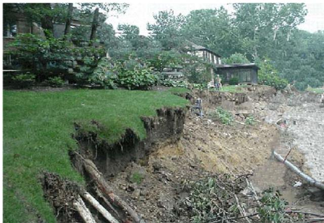
**Figure 2-11.** Property loss and sediment loading due to shoreline erosion. A healthy vegetative buffer instead of turf could help prevent this.
