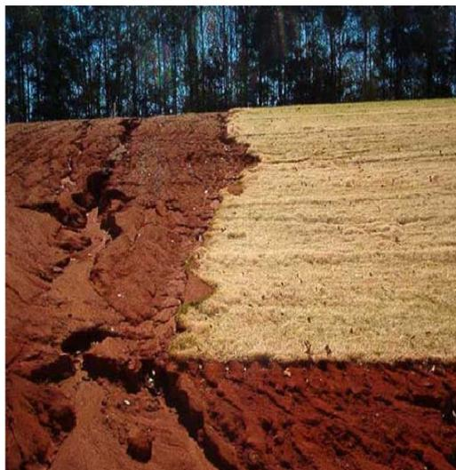
**Figure 2-13.** This comparison shows how effective mulch, within an erosion control blanket, is at preventing erosion.
